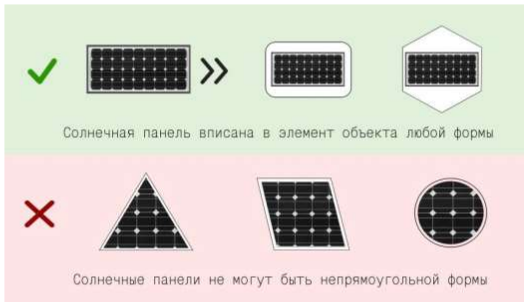
Figure 1. Installation of Energetic Energies. Solar panels have a certain shape - rectangular. In this case, polycrystalline photocells of solar panels are a rectangle or square, and monocrystalline ones are a square with beveled corners. They are more fragile, and this shape allows you to avoid a large number of defects in production - chipped corners. Solar panels on a thin-film basis can theoretically be of any
